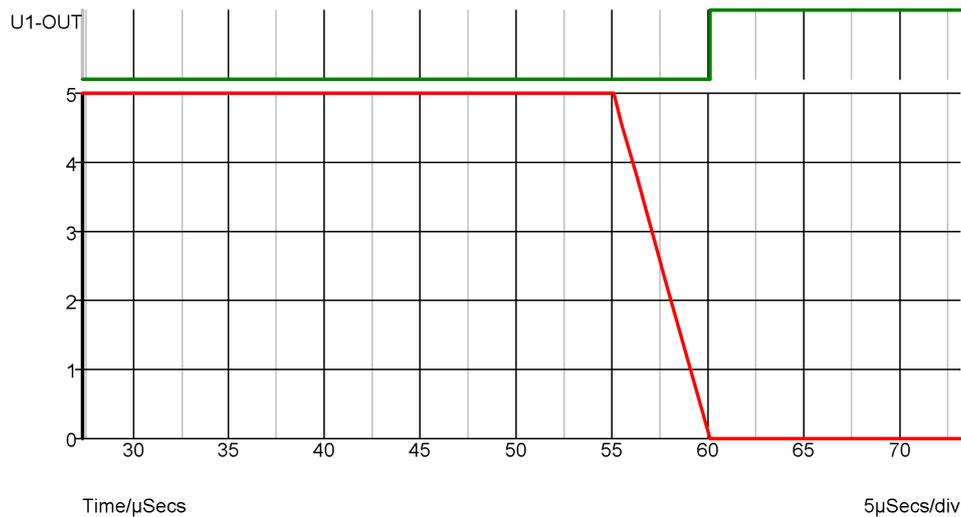
The graph shows the input and output of the NAND gate. Because the input is analog an implicit AD interface bridge will have been connected by the simulator. In the above example the parameters for this bridge have been set to:
