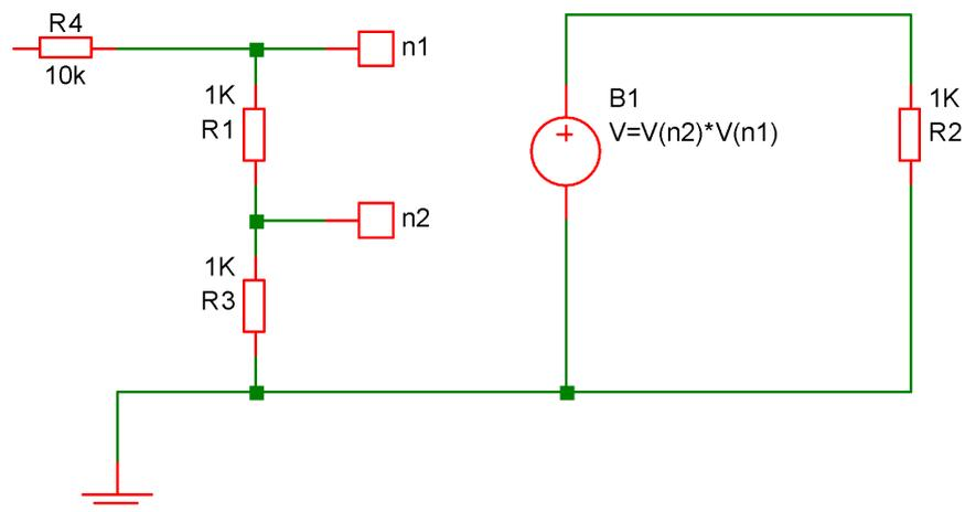
In the above circuit the voltage across B1 will be equal to the product of the voltages at nodes n1 and n2.
