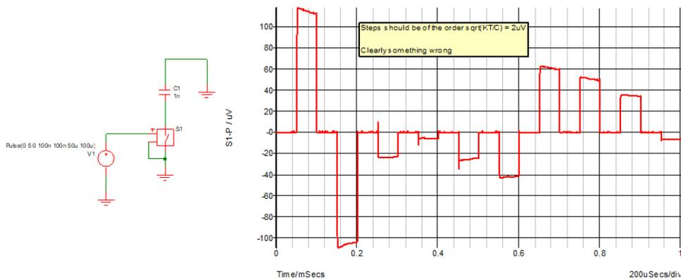
When the switch in the above circuit switches off, its conductance falls dramatically, but the noise current is set according to the on-state. This introduces gross errors as shown above.
