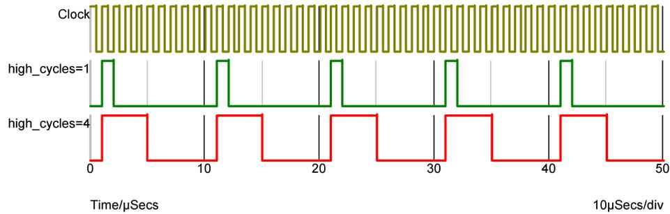
The above was carried out with `I_COUNT=0`. `I_COUNT` is the initial value of the internal counter. The output first goes high when it attains a value of 1 or `1+DIVIDE_RATIO` so when `I_COUNT` is zero (the default) the output first goes high after the first rising edge. If `I_COUNT` is set to 5 the output first goes high after the 6th rising edge and if `I_COUNT` is -20, the 21st rising edge.
