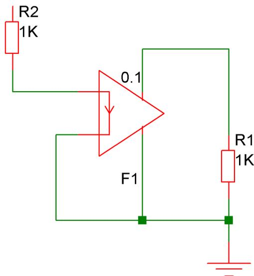
In the above circuit, the current in the output of F1 (flowing from top to bottom) will be 0.1 times the current in R2.
