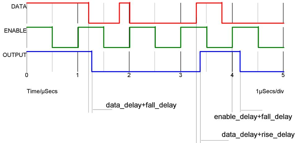
Note that any signal on the enable, set, reset or data that is shorter than the associated delay time will not be actioned. So for example, if the enable\_delay parameter is set to 10ns, a 9.9ns pulse on the enable input will not enable the latch whereas a 10.1ns pulse will enable the latch. This behaviour is the important difference between this device and the older D-type latch.
