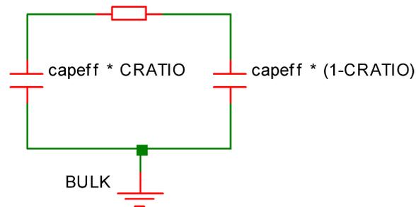
$capeff$  is the non temperature adjusted capacitance.
