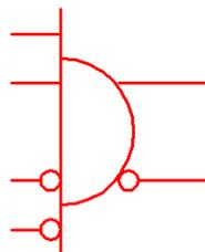
AND gate with two inverting inputs and complimentary outputs
