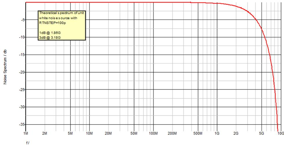
The above describes how white noise sources are implemented. It is also necessary to implement flicker noise which has a noise distribution that varies with frequency. This is done by summing multiple PWL sources with increasing step size.
