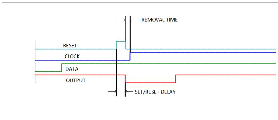
Asynchronous Set/Reset Timings
