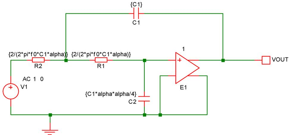
The above circuit is that of a two pole low-pass filter. C1 is fixed and  $R1=R2$ . The design equations are:
