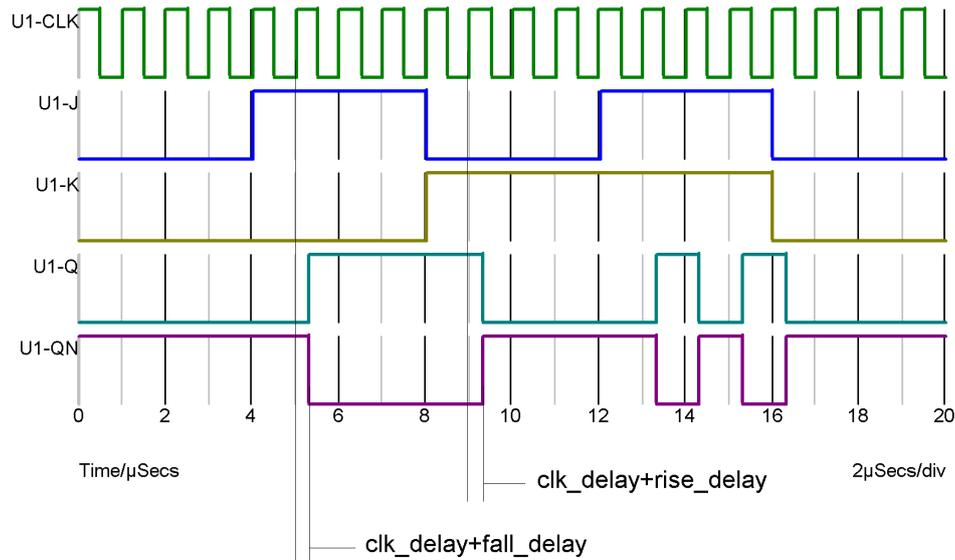
The following table describes the operation of the device when both inputs are at known states: The output can only change on a positive edge of the clock.
