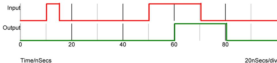
The Buffer device has an optional *stored delay* (also known as transport delay) parameter that makes possible the specification of pure delays.
