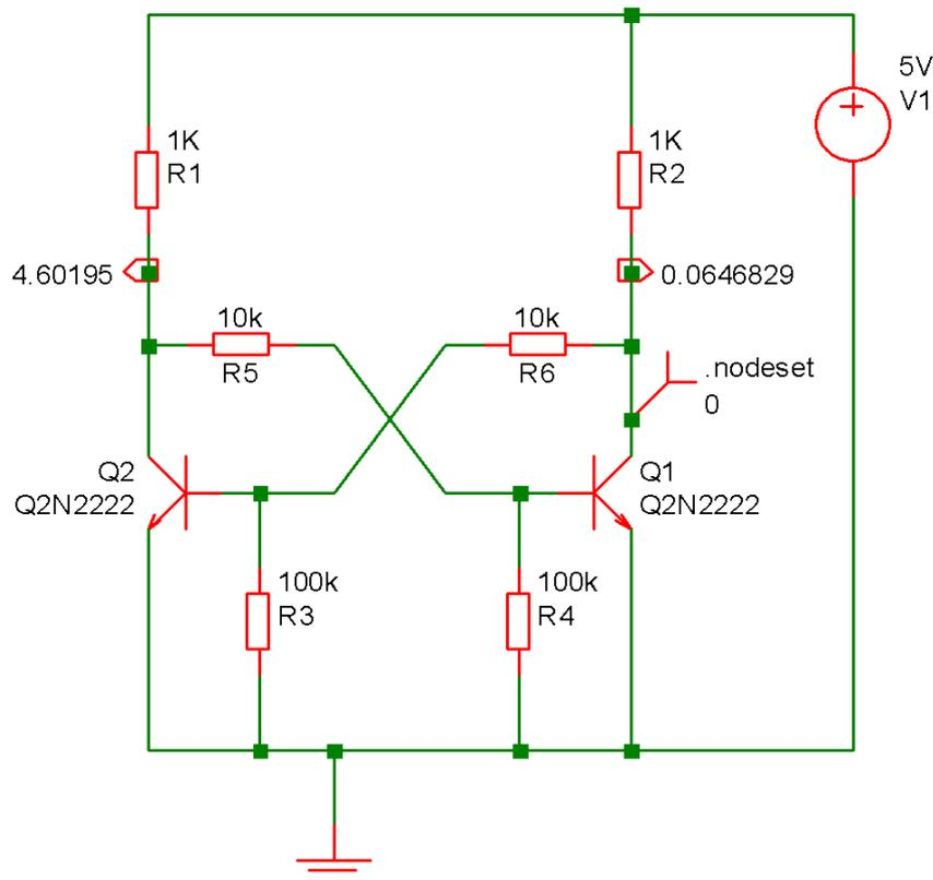
A nodeset has been applied to the collector of Q1. This has forced Q1 to be on and Q2 to be off. If the nodeset were absent the solution would actually leave both Q1 and Q2 partially on. In real life this would not be stable but it is numerically accurate.
