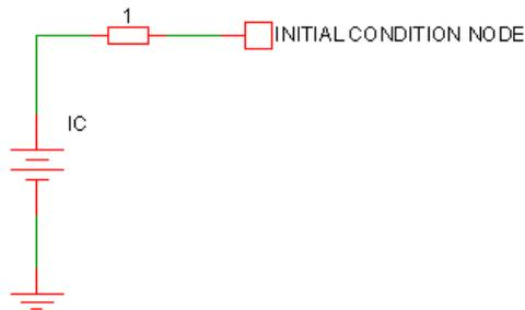
The above shows a driving resistance of  $1\Omega$ . This is the default value but can be changed using the `ICRES` option:
