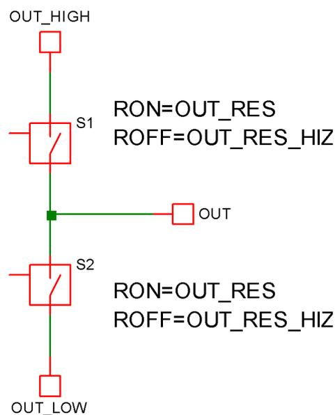
Each switch has an on state resistance of *OUT\_RES* and an off state resistance of *OUT\_RES\_HIZ*. In the logic one state, S1 is on, in the logic zero state S2 on, while in the high-impedance state, neither switch is on. When transitioning from one state to another state, each switch's resistance changes linearly to the new state's value in the time determined by the parameters *T\_RISE* and *T\_FALL*.
